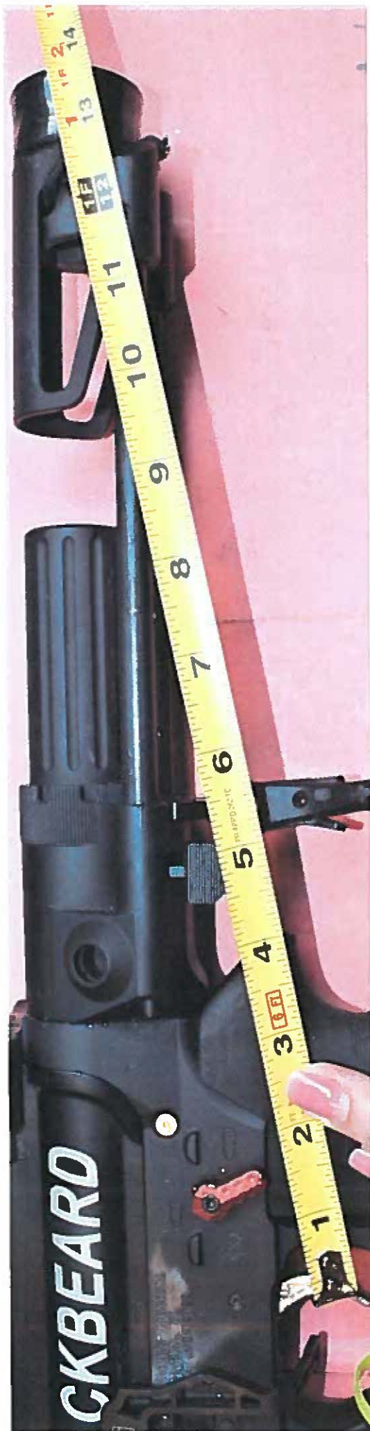
309209 - Exhibit 1 – Pictures 11 - 13: Measurement – Length of pull = approximately 13-3/4 inches.
