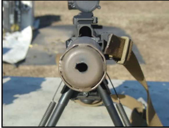
Figure 43. KAC Suppressor Baffle Strike on UUT B4
