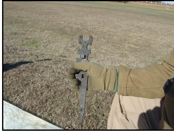
Figure 20. Tool used to remove SRM from UUTs C7-C9
